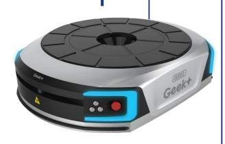
Lift Load: 1.000 kg Empty max. speed: 2 m/s
