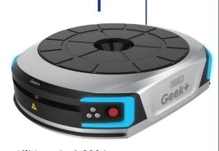
Lift Load: 1.000 kg Empty max. speed: 2 m/s
